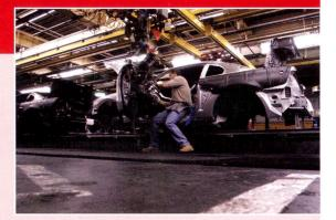
The finished body shell then goes into the paint shop where the data carrier determines the colour. In final assembly, the interior and exterior parts (for example the front and rear bumpers, headlights, windscreen, and other windows) are fitted. After quality control and a final check, the finished car can be released. It is now ready for delivery to its new owner.
