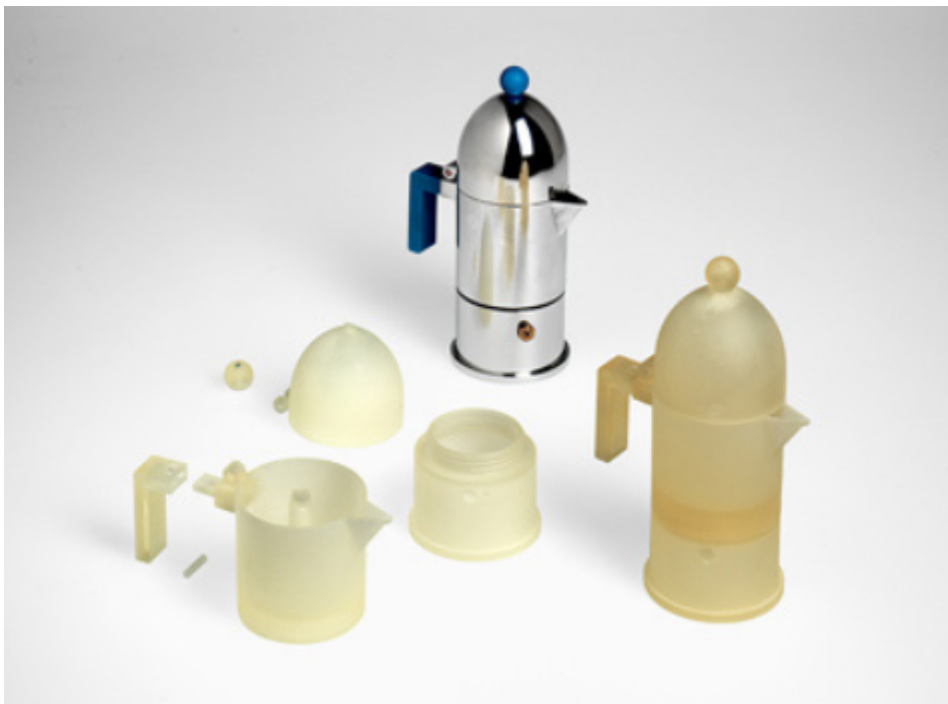
A very useful tool is 3D printing, which is only one possibility for rapid prototyping.
